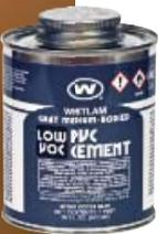
**PVC GRAY MEDIUM BODIED LOW VOC CEMENT\*** A medium set for use through 6" (15.24 cm) diameter Sch. 40 & Sch. 80 PVC pressure pipe and through 8" (20.32 cm) diameter non-pressure pipe. Meets ASTM D2564. **MADE IN THE U.S.A.**
