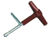
**HEAVY DUTY WATER HEATER ELEMENT WRENCH** A professional grade tool that easily removes elements without damaging the unit. Sliding "T" type handle allows for even pressure on both ends. Removes the most stubborn elements. 12 point heavy duty chrome plated steel socket and 18" (45.7 cm) "T" handle.
