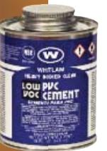
**PVC CLEAR HEAVY BODIED LOW VOC CEMENT\*** A slow set for use through 12" (30.48 cm) diameter Sch. 40 & Sch. 80 PVC pressure pipe and through 16" (40.64 cm) diameter non-pressure pipe. Meets ASTM D2564. **MADE IN THE U.S.A.**
