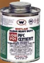
**PVC CLEAR HEAVY DUTY LOW VOC CEMENT\*** A medium set for use through 12" (30.48 cm) diameter Sch. 40 & Sch. 80 PVC pressure pipe and through 16" (40.64 cm) diameter non-pressure pipe. Meets ASTM D2564. Recommended as a One-Step Solvent Weld Cement for Drain, Waste and Vent (DWV) pipe and fittings in non-pressure applications in sizes upto 4" (10.16 cm) where acceptable by local code. **MADE IN THE U.S.A.**
