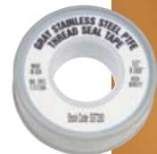
**QUALITY IMPORT PTFE TAPE** Pipe Joint Compound in Tape Form. Packed on a Spool with Cover. 3.5 Mil Thick, 0.38g/cm<sup>3</sup> Density. Meets MIL-T-27730A. Meets International Fuel Gas Code 403.9.3 for Thread Joint Compounds.
