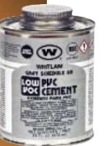
**PVC GRAY SCH. 80 HEAVY BODIED LOW VOC CEMENT\*** A slow set for use through 12" (30.48 cm) diameter Sch. 40 & Sch. 80 PVC pressure pipe and through 16" (40.64 cm) diameter non-pressure pipe. Meets ASTM D2564. **MADE IN THE U.S.A.**
