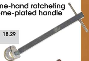
**NO HUB TORQUE WRENCH** For tightening 5/16" coupling nuts to 60 in. lbs. Automatic release at pre-set 60 in. lbs. T-Handle ratchets one way. Built-in reversing bar.
