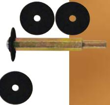
**“ZIPPY” METAL BLADE INTERNAL PLASTIC PIPE CUTTER\*** 1 each 1-1/2" (3.81 cm) diameter metal shear blade per bag with 4" (10.16 cm) long zinc plated shaft that fits 1/4" (.64 cm) or 3/8" (.95 cm) drills. For cutting 2" (5.08 cm) or larger PVC or ABS plastic pipe. **WARNING - Do not operate cutter in reverse.**
