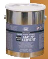
**"WEATHERPROOF" CLEAR MEDIUM BODIED WET/DRY LOW VOC PVC CEMENT\*** A fast one step\*\* cement for use on all classes and schedules of PVC pressure pipe (including Sch. 80) through 6" (15.24 cm) diameter and on non-pressure systems through 8" (20.32 cm) diameter. Meets ASTM D2564. **MADE IN THE U.S.A.**
